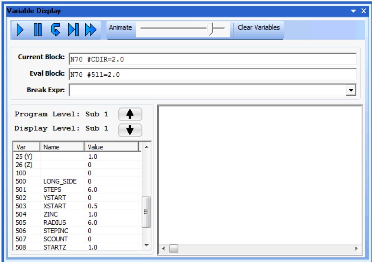
This window provides several important tools for debugging macro programs. Several controls are combined into a toolbar:
