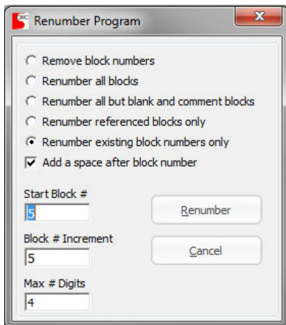
This dialog allows you to set up how you would like your program blocks to be numbered. The **Start Block #**, **Block # Increment** and **Max # Digits** settings define how the program will be numbered. If the block number exceeds the maximum digits setting then it will rollover to the starting block number.
