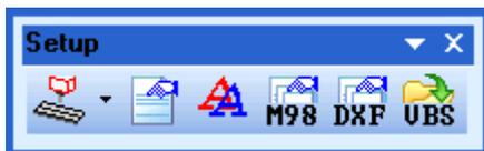
The **Setup toolbar** provides shortcuts to most of the NCPlot configuration settings including **Machine Configuration**, **Preferences**, **Address color settings**, **Subprogram settings**, and **DXF conversion settings**. It also provides quick access to your **VBS scripts**.
