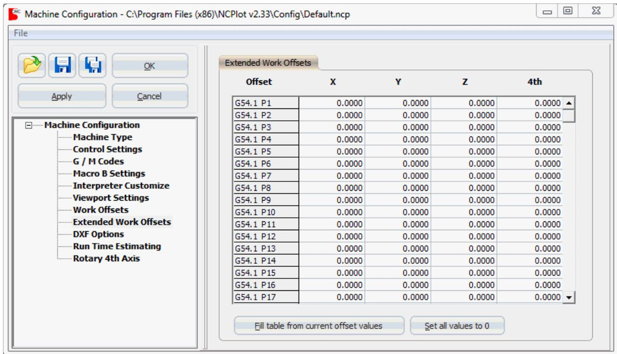
In addition to the standard work offsets G54 through G59, NCPlot also supports the use of extended work offsets. This configuration page allows the setting of your extended work offsets.
