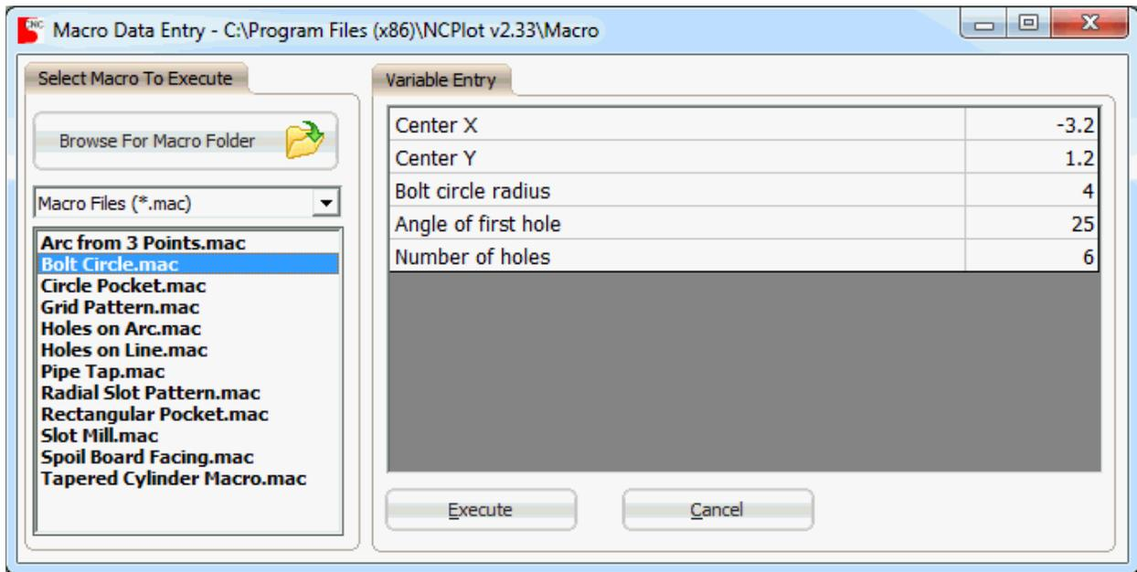
As an example, the Bolt Circle cycle asks for the X, Y center location, radius, start angle and number of holes. After this information is entered, click the "Execute" button and the resulting G-Code is inserted into your program. There are a number of cycles included with NCPlot, but you may also add your own.
