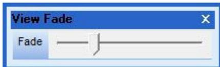
The NCPlot viewport provides View Fading, which allows you to dim the parts of the backplot that are not part of the current tool. The **View Fade toolbar** provides a slider that controls the brightness of the faded entities.
