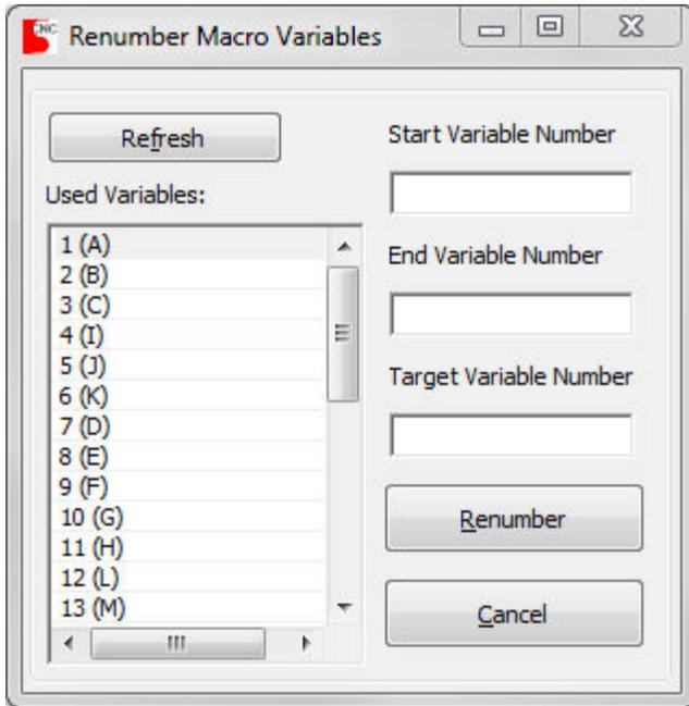
To use this tool enter the start and end variable number that you want changed as well as the target variable number then click "Renumber". The block of variable numbers from start to end are renumbered beginning at the target variable number.
