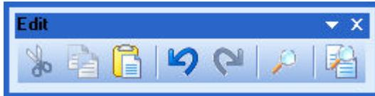
The **Edit toolbar** contains buttons for the clipboard operations cut, copy and paste as well as undo, redo, find and compare.
