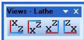
The **View toolbar** contains buttons for changing the selected viewport orientation. The displayed toolbar is dependant on the currently configured machine type. There are seven view buttons for the Mill configuration and four for Lathe.
