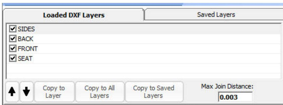
Since a drawing may contain information that you don't necessarily want converted to G-Code such as a title block or dimensions, you can turn these layers off by unchecking the box next the layer name. When layers are turned off or on the viewport will update to display just the layers that are on.
