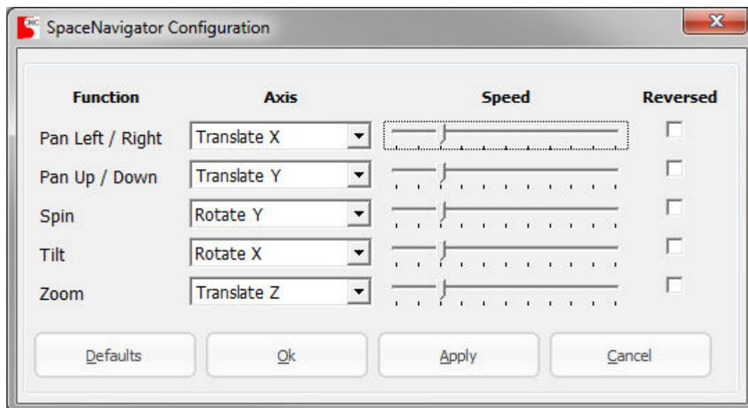
Each Function may be controlled by any one of the six device axes. You can also adjust the speed and direction for each of the functions.
