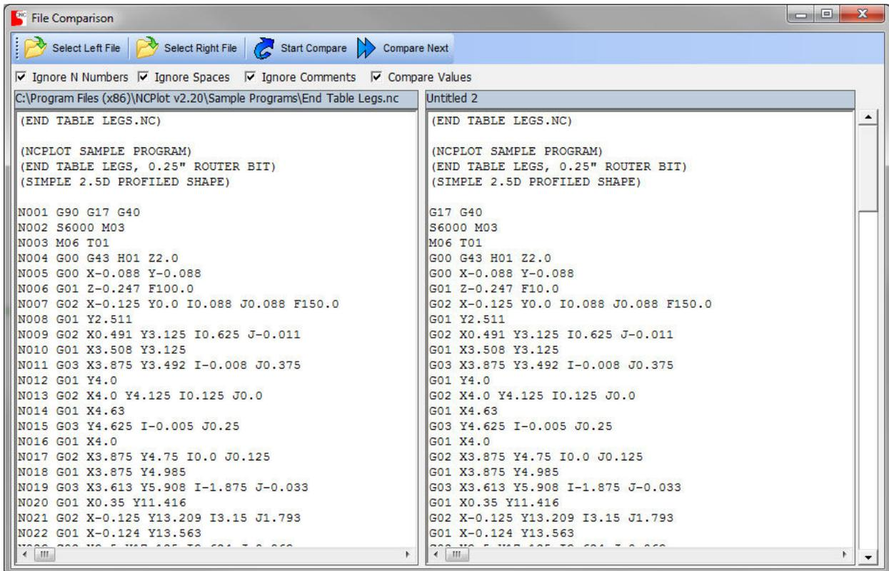
This tool allows comparing two files and highlighting any differences. It consists of a button bar, option check boxes and the two files to compare. The button bar functions are:
