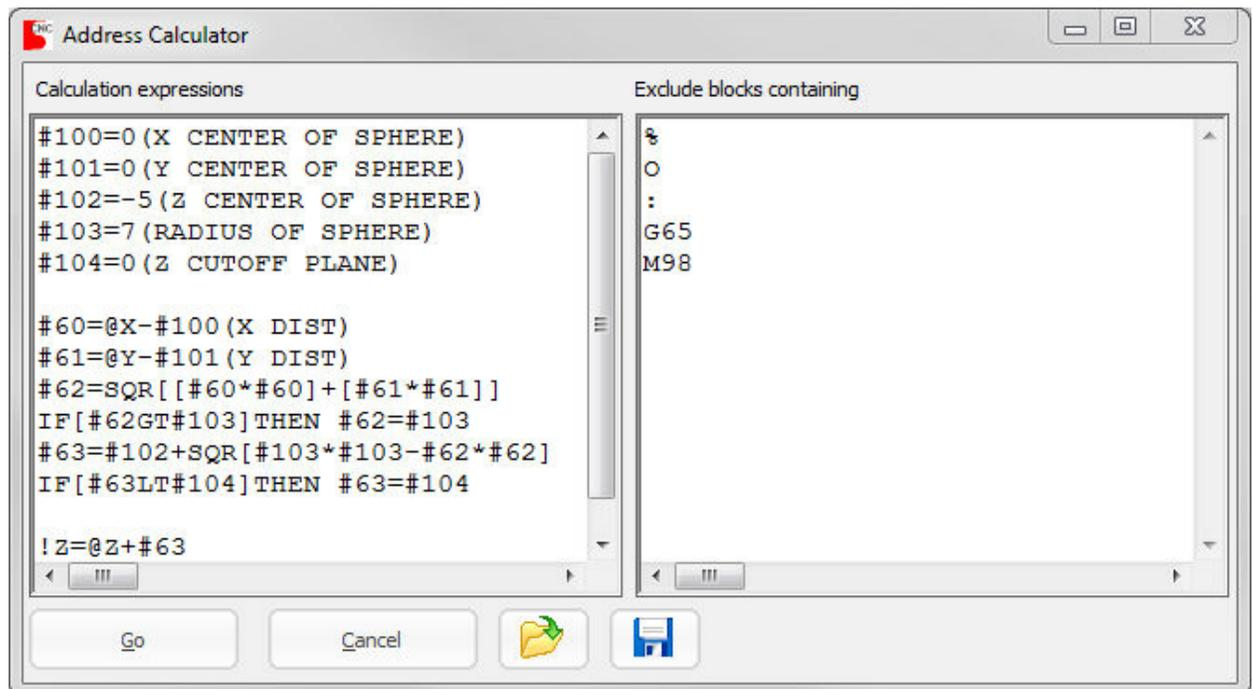
For each block in the program the address values are loaded into local variables and one or more calculation expressions can be performed. The address values can be updated based on the calculation results or even removed from the program. The expressions are given in the Macro B format and can include the "IF - THEN" macro keywords.
