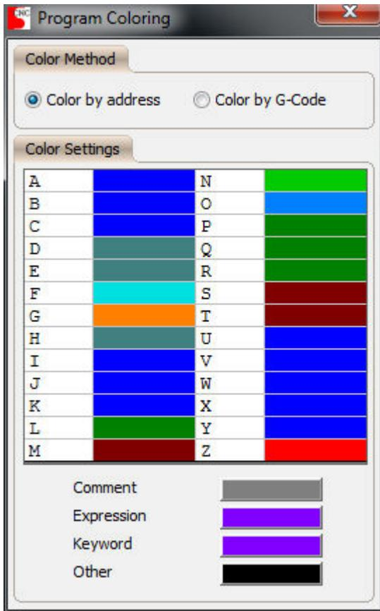
The **Color by G-Code** method applies color to each program line based on the active G-Codes. The G-Code group that is used to apply colors can be selected from the drop down list. To change the color settings, double-click the colored box next the address letter you want to change. A color picker dialog opens and you can select the color for that address. Color changes are automatically applied when coloring is enabled via the menu **Edit / Colorize**.
