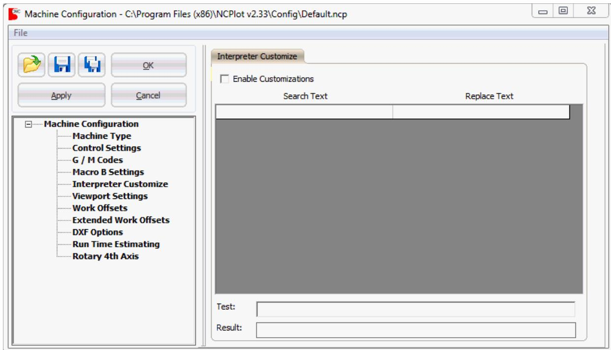
The interpreter customize page allows greater flexibility in setting up NCPlot to backplot programs that use non-standard program or G-Code formats. It does this by finding and replacing text in the program blocks before they reach the interpreter. This process does not change the program being edited, it only changes how the program is read by the backplotter.
