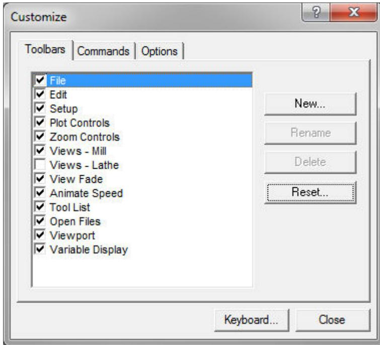
On this dialog, click the **New** button and then enter a name for the new toolbar. The toolbar is then created and will appear on the screen as an undocked toolbar. To add buttons to the new toolbar the **Customize** dialog must be left open. Click and drag buttons to move them from the other toolbars to your new toolbar, or hold the **Ctrl** key while dragging to copy them.
