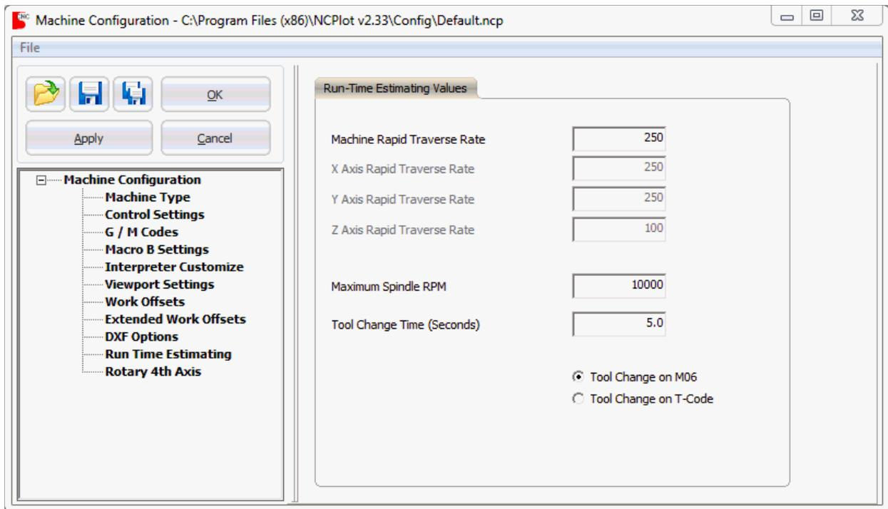
The settings on this page are used for calculating the estimated machining time of your programs. The **Machine Rapid Traverse Rate** and **Tool Change Time** settings are used for all machine types, while the **Maximum Spindle RPM** setting is used only during lathe CSS calculations.
