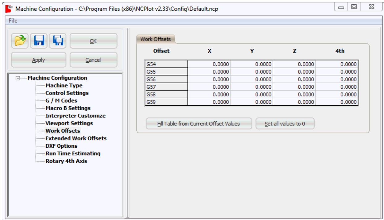
Just like your machine can accommodate multiple work offset coordinates, NCPlot can also be configured to recognize multiple work locations. This gives a backplot that accurately represents a multiple fixture setup.
