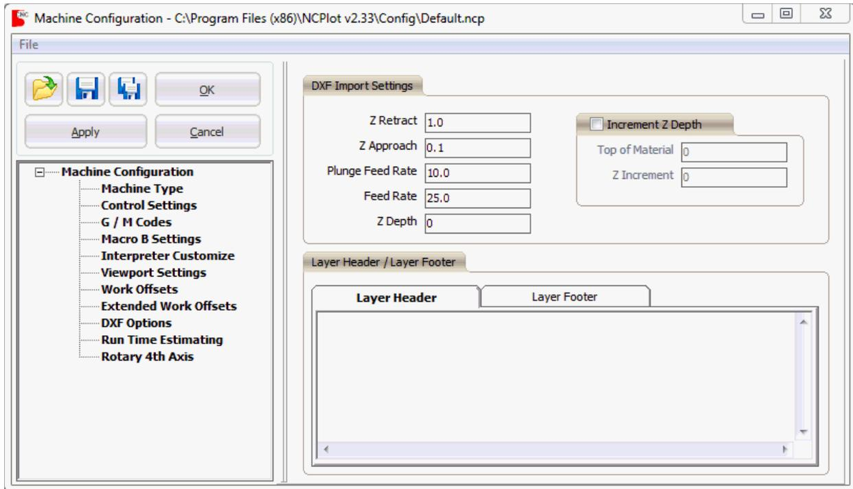
Use this page to enter default DXF drawing conversion settings. When a DXF file is loaded, any layer that is not in your saved layer list will be given these settings. For more information see the section [Converting DXF Drawing Files](#).
